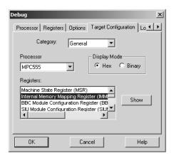
4 Click Show to open the Internal Memory Mapping Register dialog. Confirm that the **FLEN-flash enable** check box is selected as shown below.
